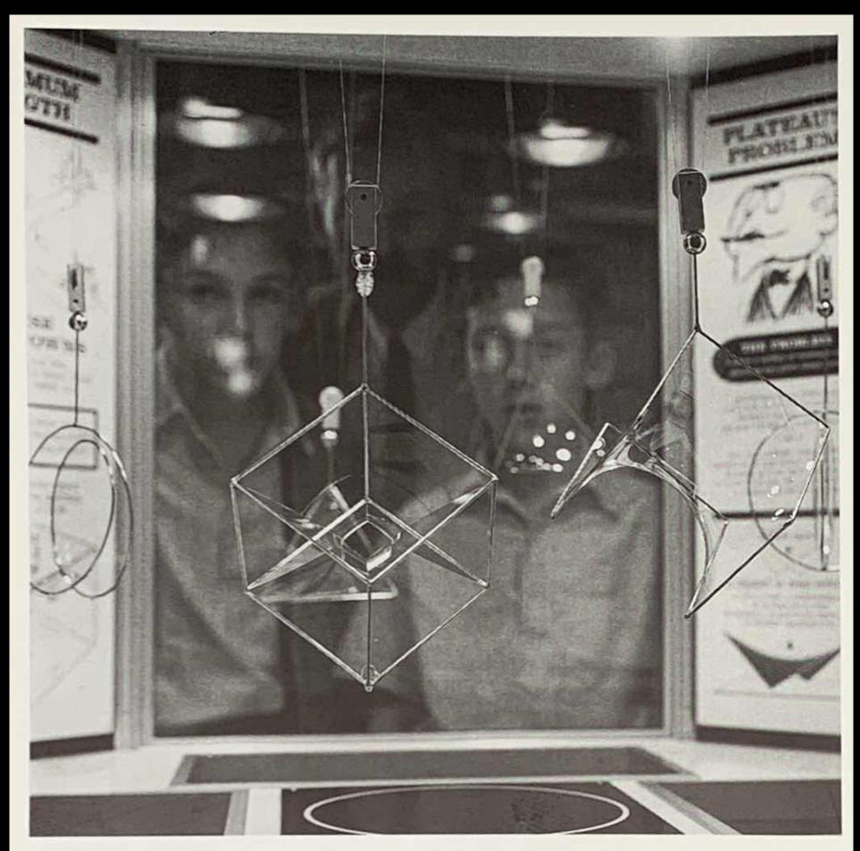
A soap-solution dipping device for demonstrating minimal surfaces
