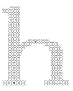
The program that is paraphrased in the text might prepare this character for a low-resolution printing device. Note the five key points numbered 1, 2, 3, 4, and 5; the center of the 'pen' travels through these points as it draws the letter.
